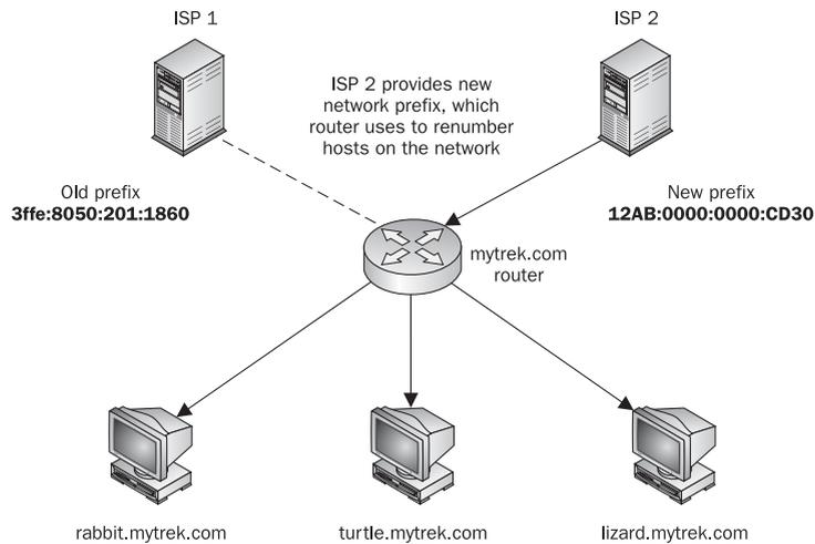
**FIGURE 35-2** Router renumbering with IPv6 autoconfiguration
