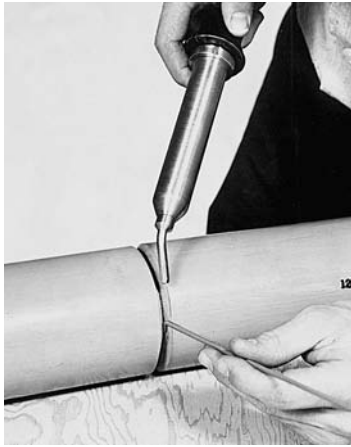
FIGURE 34-9 Using a hot-gas torch to make a weld in plastic pipe.
