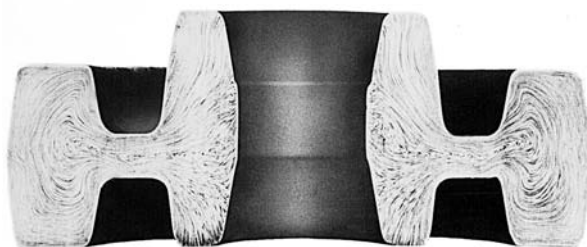
FIGURE 15-4 Flow structure of a hot-forged gear blank. Note how flow is parallel to all critical surfaces. (Courtesy of Bethlehem Steel Corporation, Bethlehem, PA.)
