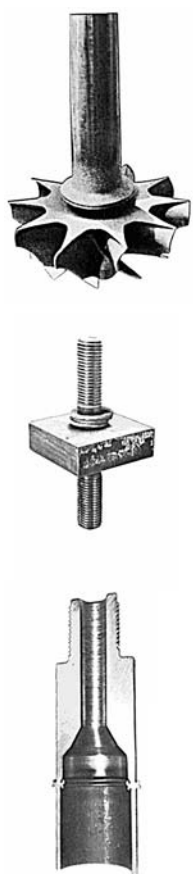
FIGURE 32-17 Some typical friction-welded parts. (Top) Impeller made by joining a chrome-moly steel shaft to a nickel-steel casting. (Center) Stud plate with two mild steel studs joined to a square plate. (Bottom) Tube component where a turned segment is joined to medium-carbon steel tubing. (Courtesy of Newcor Bay City, Division of Newcor, Inc., Royal Oak, MI.)
