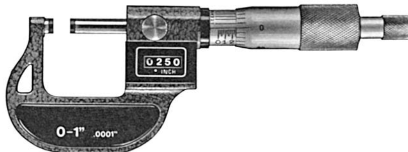
FIGURE 10-20 Digital micrometer for measurements from 0 to 1 in., in 0.0001-in. graduations.
