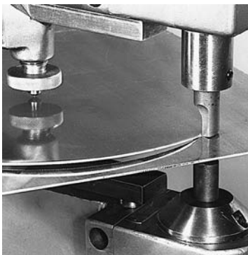
FIGURE 17-9 Shearing operation being performed on a nibbling machine. (Courtesy of Pacific Press Technologies, Mt. Carmel, IL.)
