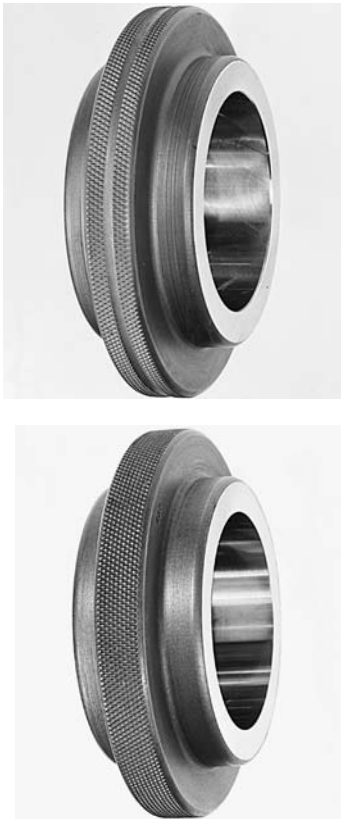
FIGURE 10-36 Go and no-go (on right) ring gages for checking a shaft. (Courtesy of Automation and Measurement Division, Bendix Corporation.)
