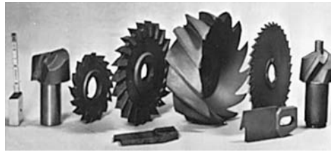
FIGURE 12-27 Group of intricate cutters produced by ceramic mold casting. (Courtesy of Avnet Shaw Division of Avnet, Inc., Phoenix, AZ)
