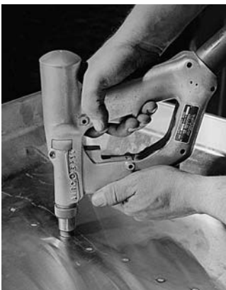
FIGURE 31-22 Making a spot weld by the inert-gas-shielded tungsten arc process. (Courtesy of Air Reduction Company Inc., New York, NY)
