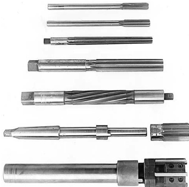
FIGURE 23-23 Types of reamers: (top to bottom) Straight-fluted rose reamer, straight-fluted chucking reamer, straight-fluted taper reamer, straight-fluted hand reamer, expansion reamer, shell reamer, adjustable insert-blade reamer.
