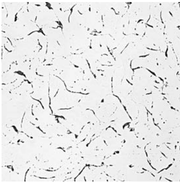
FIGURE 4-16 Photomicrograph of typical gray cast iron; 1000X. (Courtesy of Bethlehem Steel Corporation, Bethlehem, PA.)
