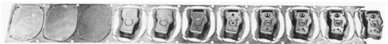
FIGURE 17-17 The various stages of an 11-station progressive die. (Courtesy of the Minster Machine Company, Minster, OH.)
