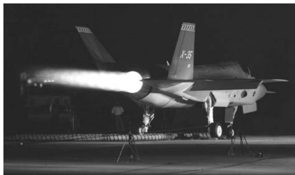
FIGURE 7-5 Superalloys and refractory metals are needed to withstand the high temperatures of jet engine exhaust. (Courtesy of Northrop Grumman Corporation, Los Angeles, CA.)
