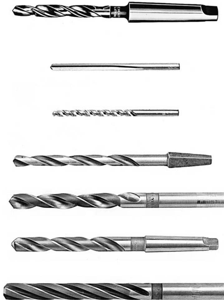
FIGURE 23-3 Types of twist drills and shanks. Bottom to top: Straight-shank, three-flute core drill; straight-shank; taper-shank; bit-shank; straight-shank, high-helix angle; straight-shank, straight-flute; taper-shank, subland drill.
