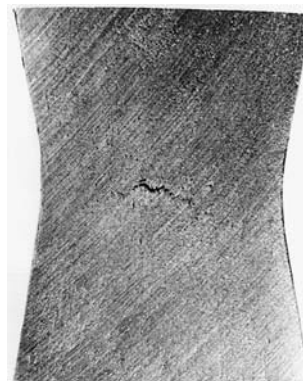
FIGURE 2-11 Section of a tensile test specimen stopped just prior to failure, showing a crack already started in the necked region. (Courtesy of E. R. Parker.)
