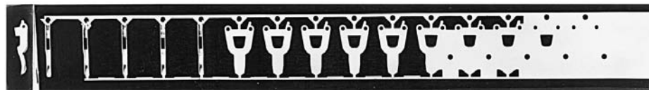
FIGURE 17-66 Example of the piercing, blanking, and forming operations performed on a multislide machine. (Courtesy of U.S. Baird Corporation, Stratford, CT.)
