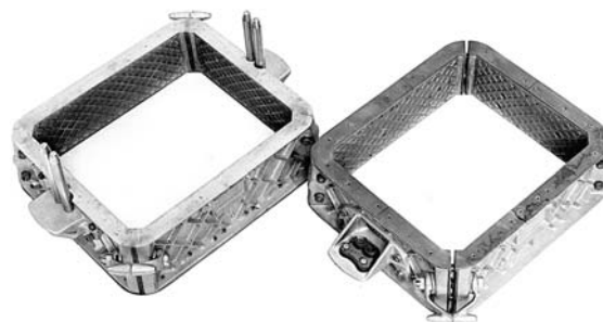
FIGURE 12-11 Bottom and top halves of a snap flask. (Left) drag segment in closed position; (right) cope segment with latches opened for easy removal.
