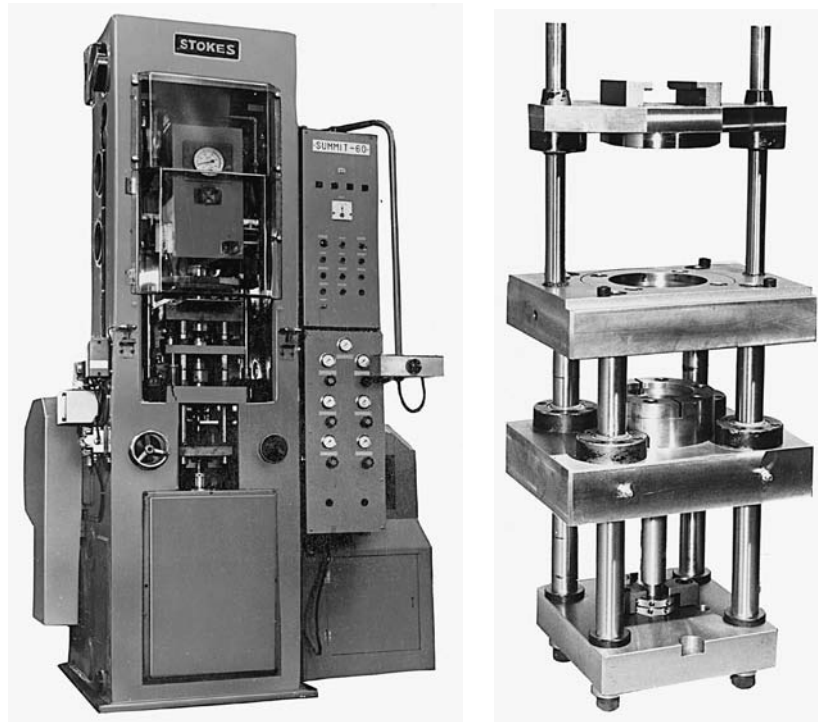
FIGURE 18-3 (Left) Typical press for the compacting of metal powders. A removable die set (right) allows the machine to be producing parts with one die set while another is being fitted to produce a second product. (Courtesy of Alfa Laval, Inc., Warminster, PA.)
