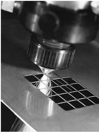
FIGURE 31-27 Cutting sheet metal with a plasma torch. (Courtesy of GTE Sylvania, Danvers, MA)
