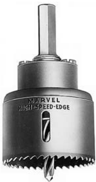
FIGURE 23-9 Hole cutter used for thin sheets. (Courtesy of Armstrong-Blum Manufacturing Company.)
