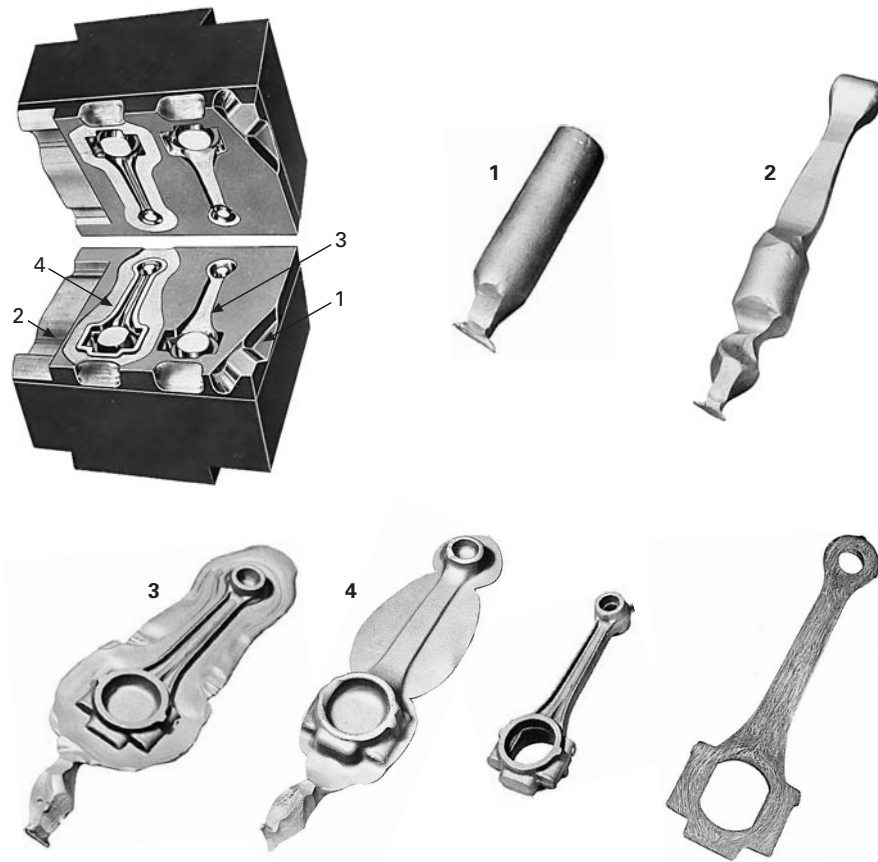
FIGURE 16-12 Impression drop-forging dies and the product resulting from each impression. The flash is trimmed from the finished connecting rod in a separate trimming die. The sectional view shows the grain flow resulting from the forging process. (Courtesy of Forging Industry Association, Cleveland, OH.)
