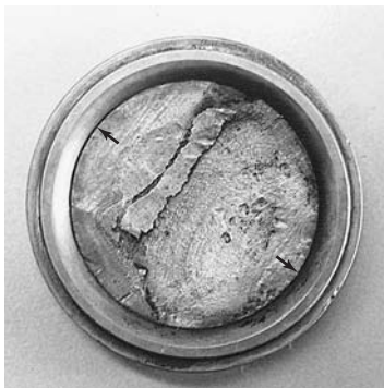
FIGURE 2-28 Progressive fracture of an axle within a ball-bearing ring, starting at two points (arrows).
