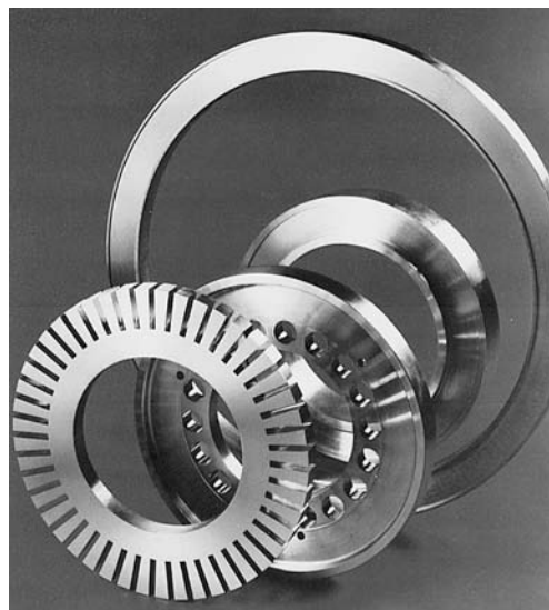
FIGURE 13-10 Electrical products (collector rings, slip rings, and rotor end rings) that have been centrifugally cast from aluminum and copper. (Courtesy of The Electric Materials Company, North East, PA.)
