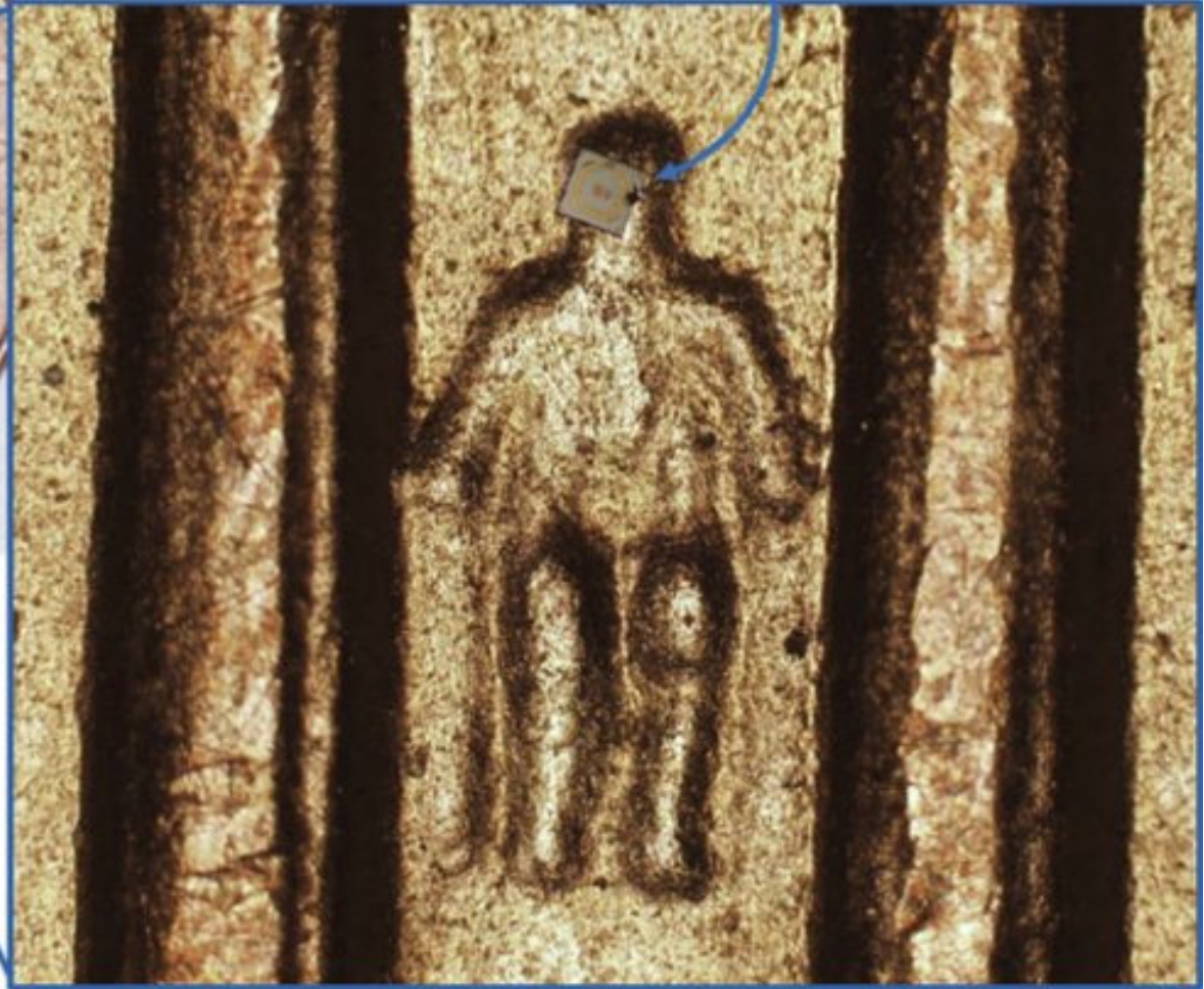
28.8: A 5.8GHz Power-Harvesting 116 \mu m x 116 \mu m "Dielet" Near-Field Radio with On-Chip Coil Antenna
